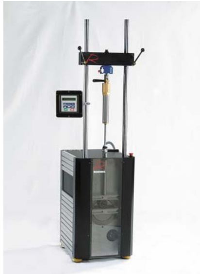
Figure 5.0 A crank dynamometer from Roehrig.
