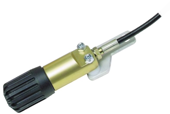
Figure 29.0 Hydraulic spring preload adjuster knob.
